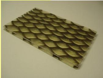
YST (You See Through) is a transparent sandwich panel with a honeycomb structure. YST panels are produced on customer demand. The honeycomb structure is covered on both sides with a 1.5mm thick layer of GRP (glass reinforced polyester), Finished with an all weather resistant coating so they are fit for outdoor use.
