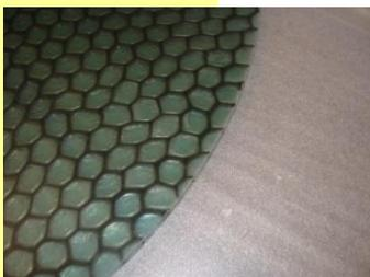
The YST standard panel has a uniform honeycomb structure. Depending on the wanted look and feel the cells are made of aluminum or cardboard. The cell size comes in different measures. Most commonly used is 20-25mm. The maximum size of the YST standard panel is 3000 x 1200mm. Thickness is usually 15mm but other dimensions are of course possible
