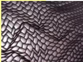
As in the standard panel, also the cell measurements in the YST Organic are variable. A usual size is 20-25mm
